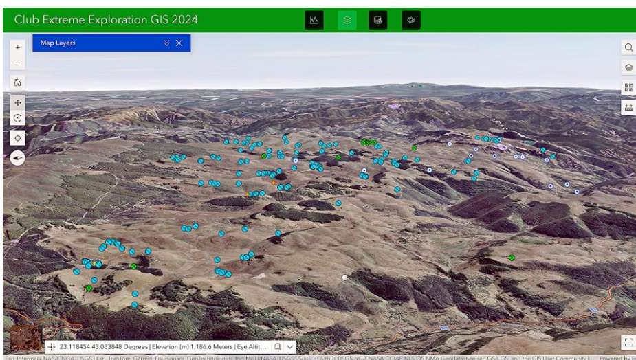
3D GIS of the exploration area With dig entrances(blue), cave entrances(green), sinkholes(yellow) and springs(blue) Basemap: orthophoto 2011
