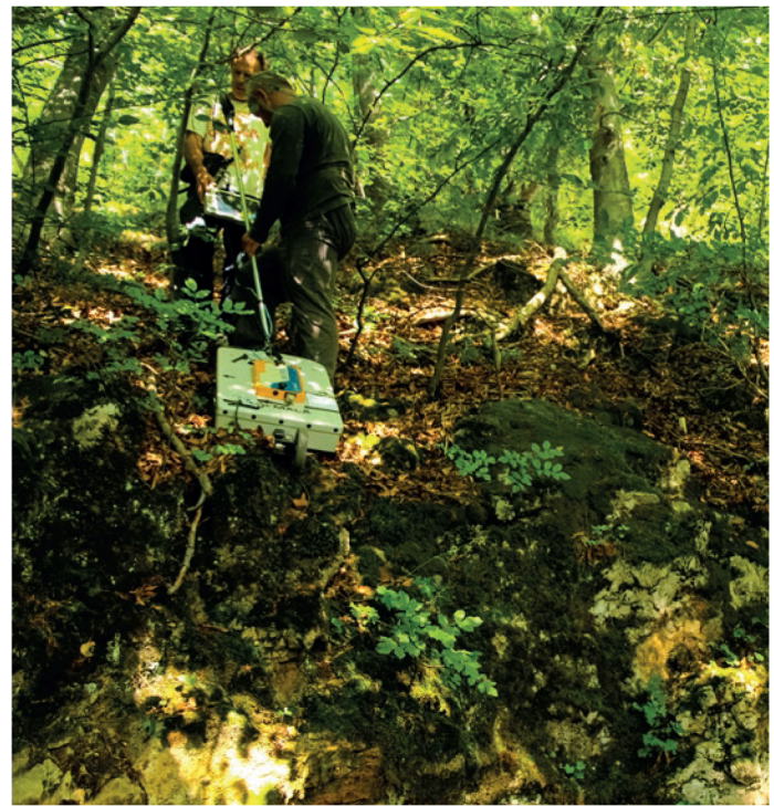
▲ Figure 4, GPR measurements just above the cave entrance.
