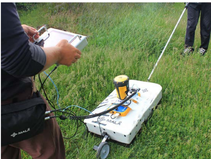
Typical GPR Configuration with 250MHz Shielded Antenna
